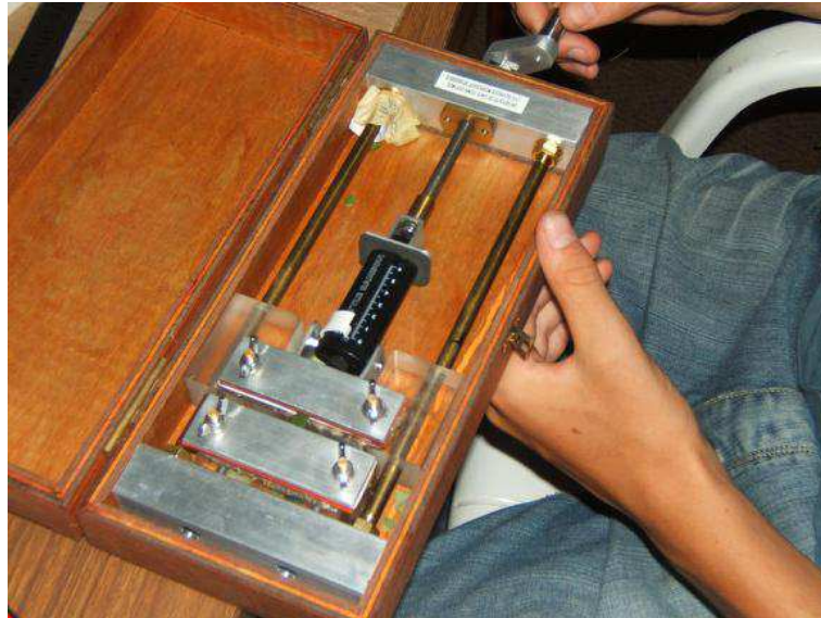
Figure A.2: Custom-built device for measuring leaf tensile strength.
